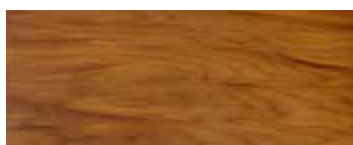
KAURI LEVGATO · MACHINE SANDED KAURI · KAURI MASCHINELL GESCHLIFFEN KAURI PONCÉ · KAURI LLJADO A MÁQUINA
