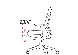
7 different positions. Depth adjustment with self-return mechanism
